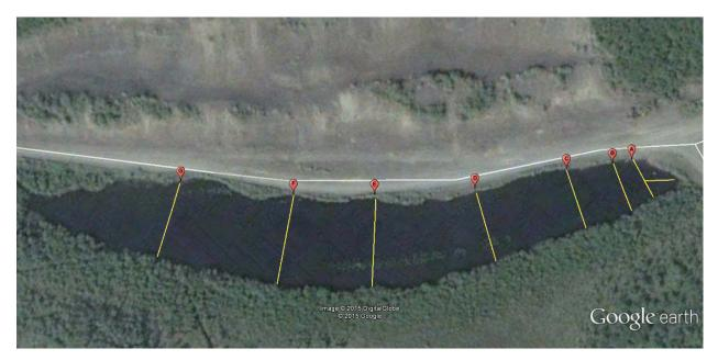
Figure 1. Transects A-G with start locations (at the letters) and approximate track and end locations. Transect A had a side portion to cover the shallow end of the lake where debris was noted from shoreline observations.
